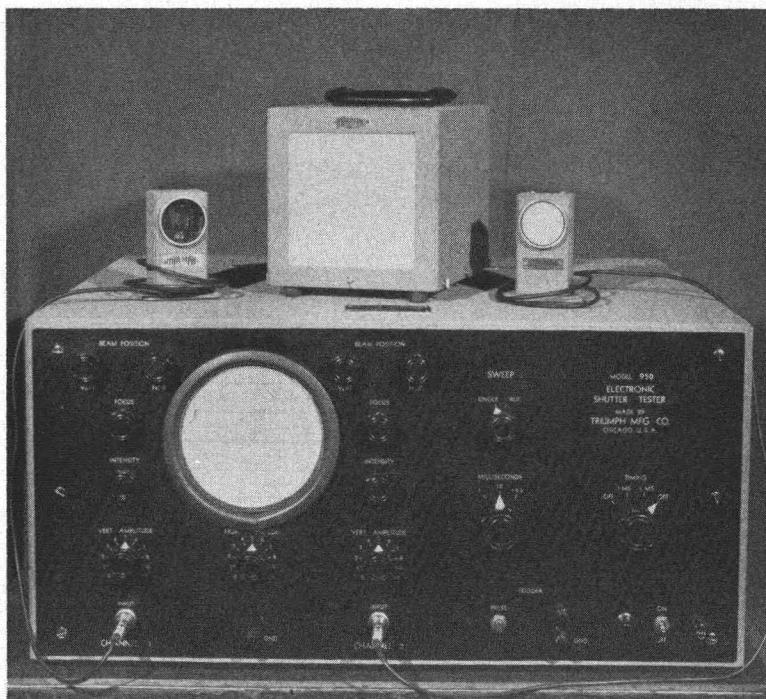
FIG. 1. Electronic shutter analyzer (tester) including the light box and two phototubes.
