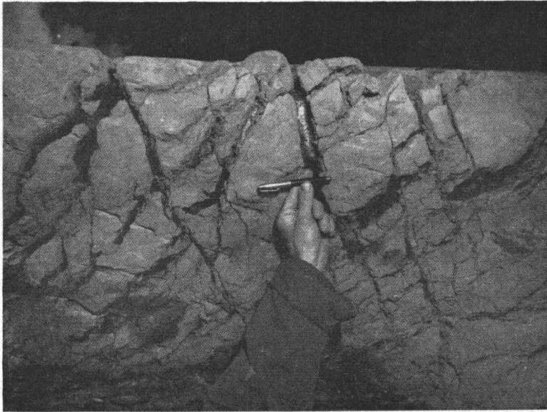
FIG. 13. This shows lenses of ice in frozen fine sand with silt.
