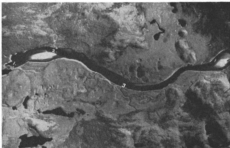
FIG. 7. A stretch of river showing various obstacles to driving pulpwood: (1) Rocks; (2) Shoal; (3) Low banks.
