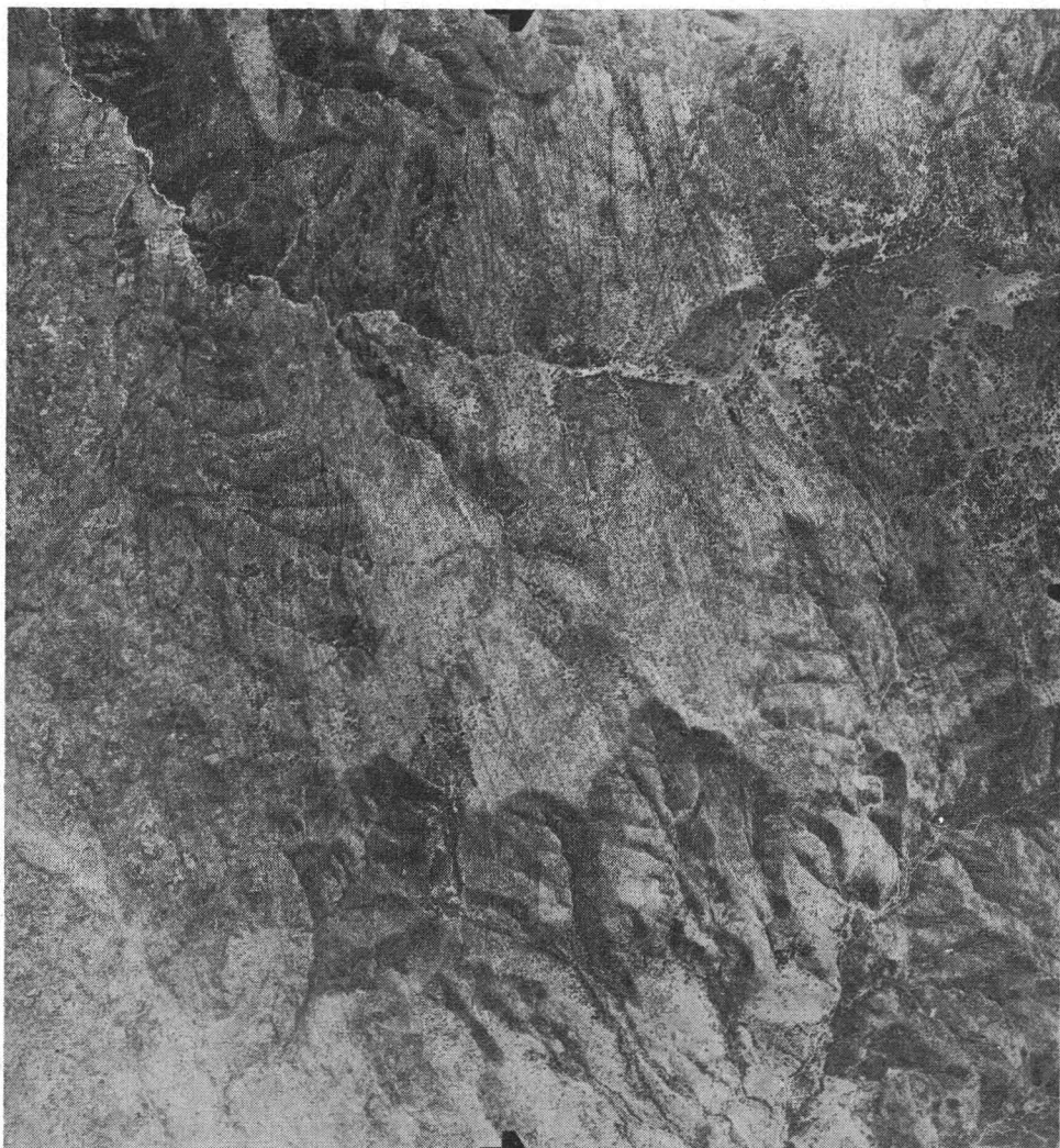
FIG. 7. Stress patterns (indicated by the numerous small dark lines of color and vegetation running from top to bottom) that may be related to the intrusion of igneous rock appearing in the upper right portion of the photo. This area, while possessing a somewhat different appearance due to vegetative and tonal differences, is most easily distinguished by its difference in land form. This is easily seen through a stereoscope though it is not at all apparent here.
