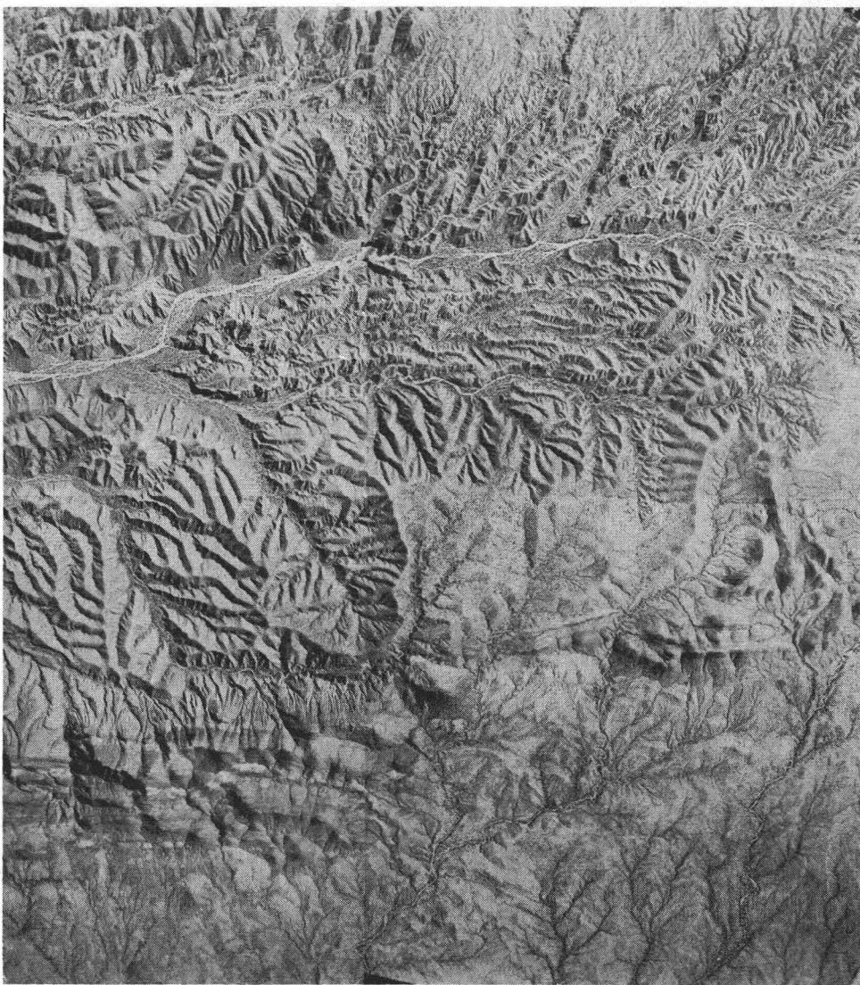
FIG. 2. An illustration of the varying response to arid weathering exhibited by earth and rock materials of varied characteristics. At least five, and possibly six, materials can be distinguished together with their boundaries, by separating them on the basis of surface drainage patterns alone. Note the sedimentaries that stand out boldly in the lower part of the picture.
