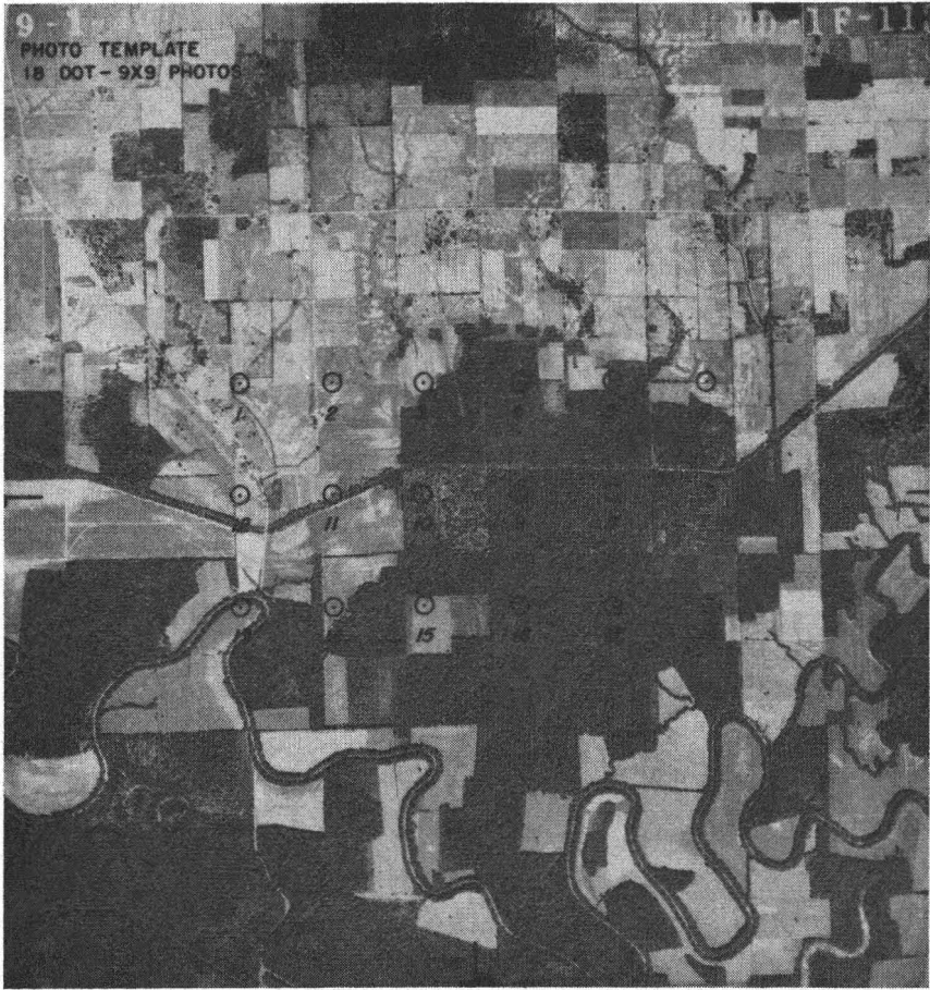
FIG. 5. Transparent templet oriented over each contact print marks the plots to be classified. Only a fraction of the total area is actually classified, but the resulting data will meet the standard of accuracy for most forest surveys, and can be secured far cheaper than by normal mapping procedures.
