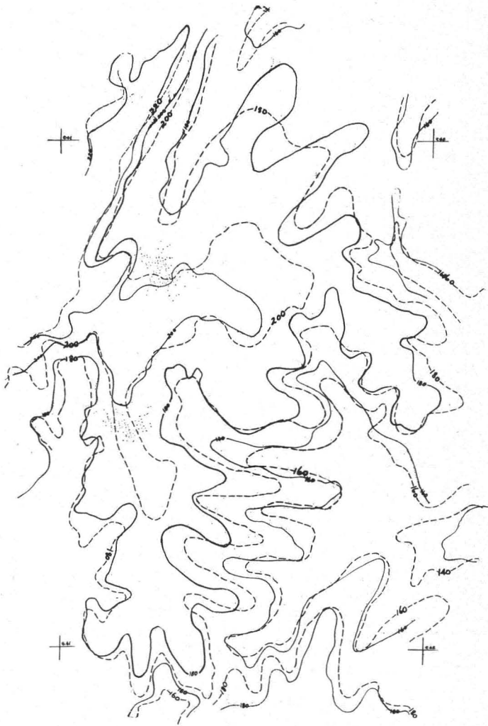
FIG. 2. Contouring of Forested Areas: Comparison of two machine tests of the same area made by independent operators.
