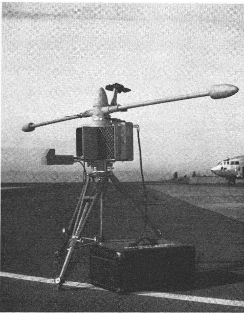
FIG. 1. The Fairchild Model IV A Analyzer with its portable power supply and transmitter case.
