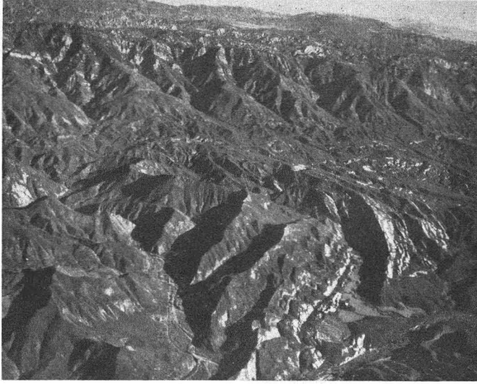
FIG. 9. Anticlinal structure and plunge of fold shown by helicopter reconnaissance of an area.
