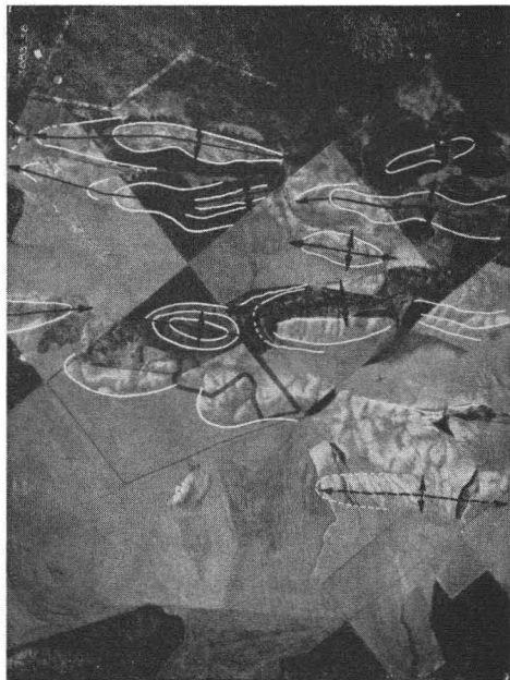
FIG. 1. Folded structures revealed by aerial photographs in area of no outcrops.
