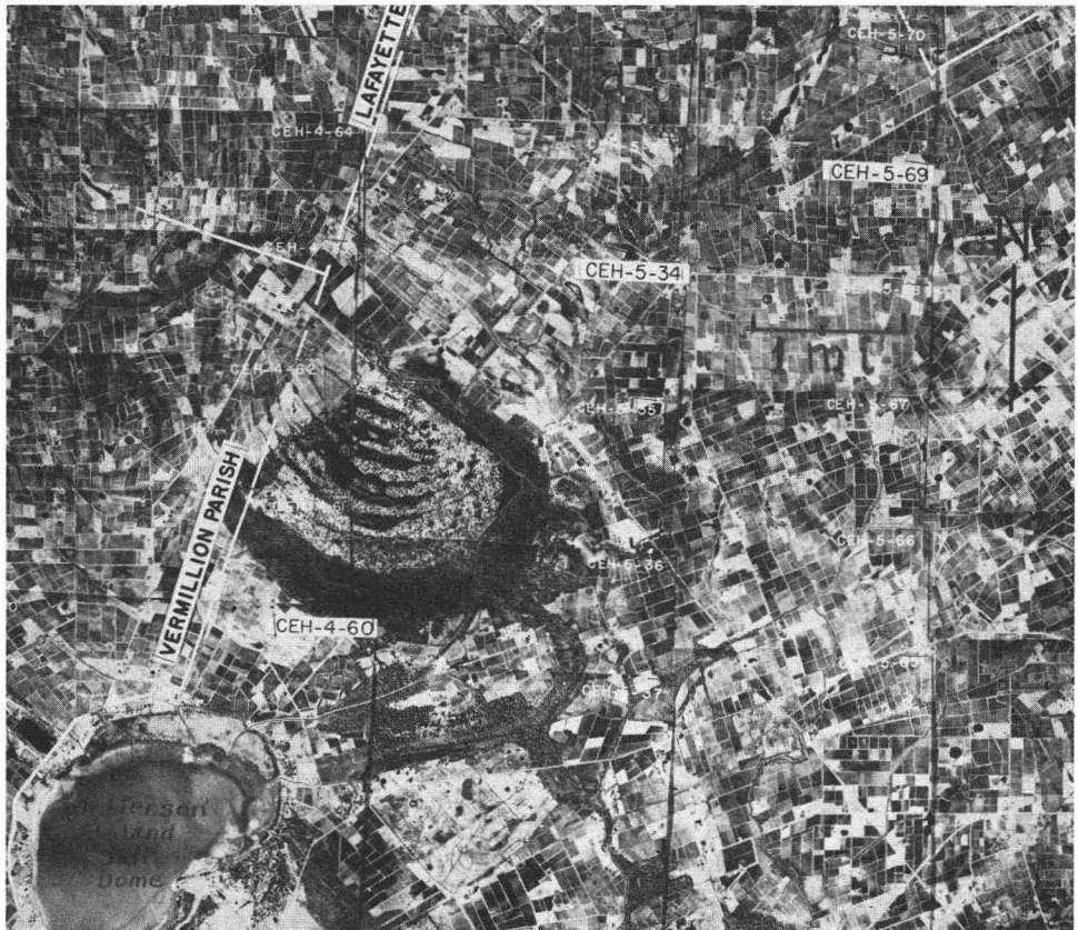
FIG. 7.—A portion of a photo-index sheet showing a small area in northwestern Iberia Parish, Louisiana. The Jefferson Island Salt Dome underlies the lake at the southwest corner of the photograph. Subsidence in the area marginal to the dome is probably responsible for the preservation of the unusual meander-loop and meander-bars that are to be seen about one to three miles to the northeast of the lake. Such meander-loops and meander-bars were very common on this late Pleistocene marine terrace at an earlier date. The preservation of this one is no doubt due to its accidental protection from erosion through subsidence. Photograph by the Commodity Stabilization Service, U. S. Department of Agriculture, Washington, D. C.
