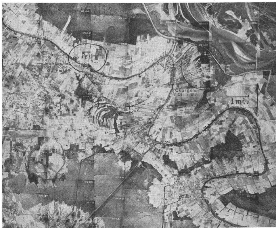
FIG. 8.—This is a portion of a photo-index sheet near the northwestern corner of St. Mary Parish, Louisiana. The sediments which underlie this surface are natural levees of Bayou Teche and sediments of the deltaic plain. Bayou Teche makes an unusually abrupt turn just northeast of the center and near the Charenton oil field. This is fairly typical of river behavior where a slight difference in the over-all resistance of sediments or rocks to weathering and erosion interrupts the otherwise more or less uniform resistance to meandering which rivers encounter. Recent elevation of the Charenton area may have contributed to this abrupt river turning. The Jeanerette Salt Dome field is present about six miles to the west of the Charenton field must north of Bayou Teche. Surface indications of the presence of this salt dome structure are less evident than in the case of the Charenton structure but are present even here in the slight indications of subsidence to the south, to the northeast, and to the northwest. Photograph by the Commodity Stabilization Service of the U. S. Department of Agriculture, Washington, D. C.
