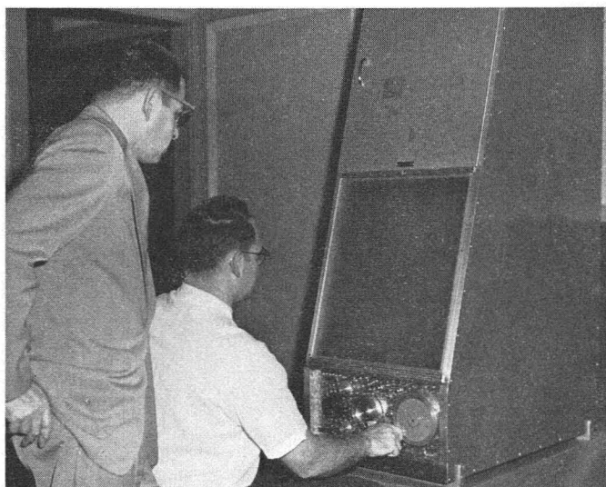
FIG. 1. This experimental table-top size stereo-projector developed for the U. S. Navy, permits two or more viewers to study a stereo-model projected on the ground glass screen.
