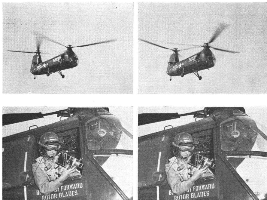
FIG. 2.—Stereograms of Piasecki helicopter, model HUP-2, and photographic equipment used in taking motion picture photography. Note use of goggles, intercommunication equipment, and "pistol grip" handle on movie camera, as discussed in text.
