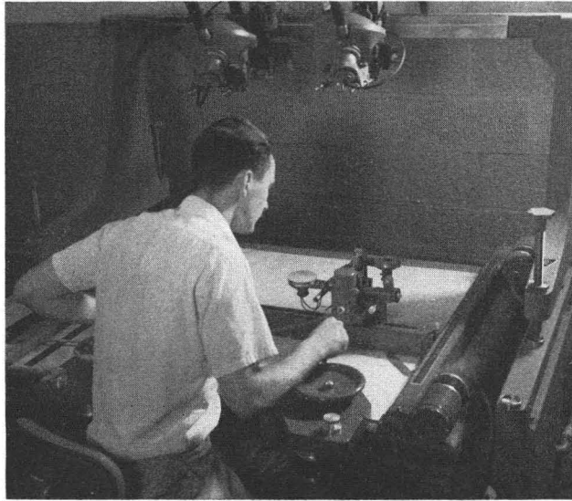
FIG. 3. The Nistri Coordinatometer shown on the Balplex Plotter. This unit is used to obtain the x , y , and z coordinates of points. It is also used on the Kelsh Plotter.
