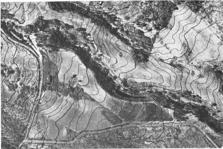
FIG. 2. Section of Photo-Contour Map covering same area as Figure 1. Note, however, that in Figure 2 the contours track properly over the entire map. This is because the photographic perspective is rectified by zones as described in this paper and becomes for practical purposes an orthographic projection at the same scale as the contour plotting.
