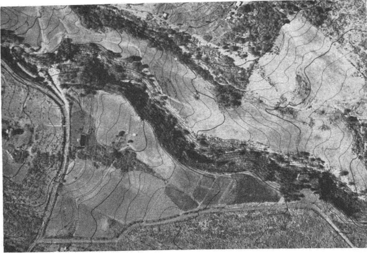
FIG. 1. Section of Mosaic map. Note how contours fail to track the road image properly becoming progressively worse to the right of the figure. This is because the contours are correctly plotted to an orthographic projection, while the planimetric detail is from a photographic perspective. The two cannot be made to agree where there is a significant ground elevation differential in the area.
