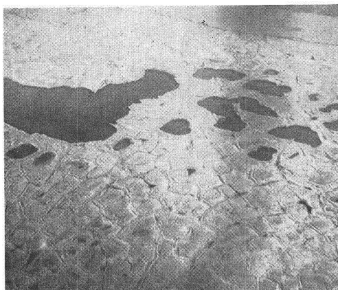
FIG. 10. Low-oblique of non-sorted polygons (ice-wedge polygons) on Arctic coastal plain near Point Barrow, in the continuous-permafrost zone, Alaska. Flat tundra surface. Part of a great thaw lake at top, angled thaw ponds (high center). Most of the polygons are high-centered, separated by shallow troughs. In left foreground and right center there are several low-center polygons with ponds developing in their center. (Photo by the author.)
