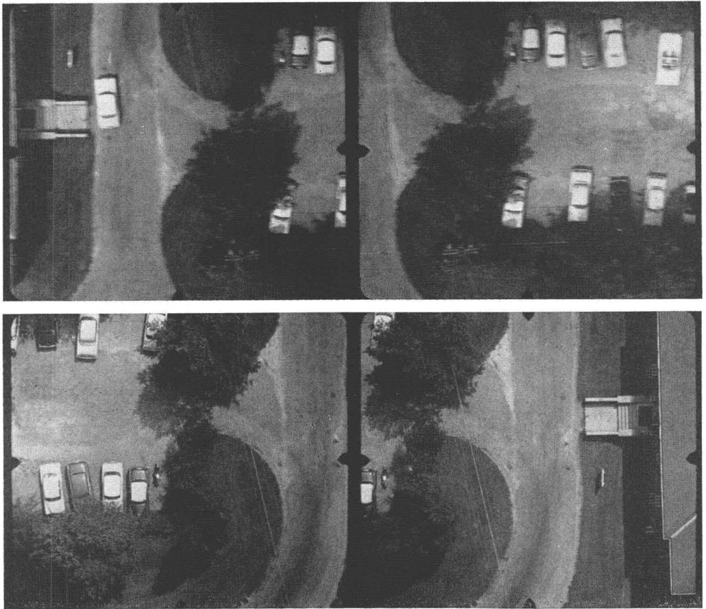
FIG. 1. 70-mm. stereo pairs of a parking lot. Upper pair was blurred by excessive image motion (shutter speed, 1/200 second). Image-motion was eliminated on lower pair by using a high-speed shutter (1/1,000) Scale 1:500.
