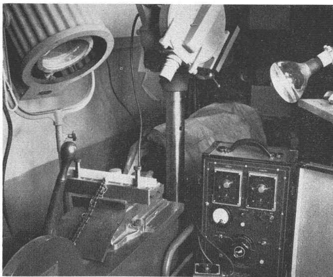
FIG. 1. High-speed motion picture equipment set up to photograph the action in the U. S. Forest Products Laboratory toughness test.
