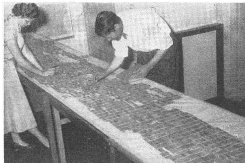
FIG. 2. Completed reference map covered with a network of colored rectangles, indicating the cost for the construction of a 380 KV power transmission line.
