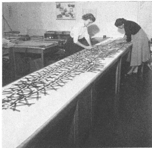
FIG. 1. Assembly of star templates for obtaining a system of control points for mapping on a skeleton map in accordance with the mechanical radial triangulation method.
