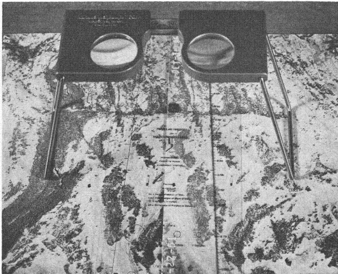
FIG. 1. Parallax wedge, printed on film, is based on the floating line principle, and is easily moved aside when other measuring devices must be used. Its initial cost is about $1.
