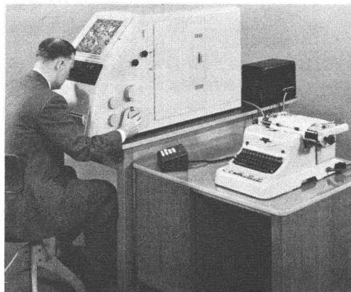
FIG. 1. The new Zeiss stereocomparator.
