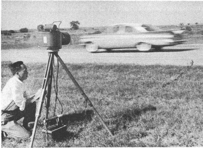
FIG. 1. Camera used for making side-view photographs of passenger cars.
