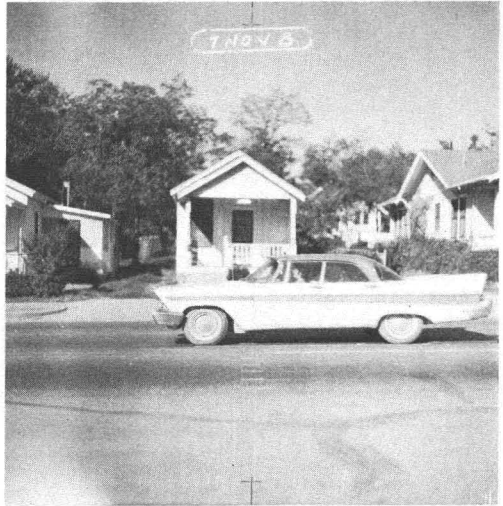
FIG. 2. Reduction of contact print of a photographic negative used for driver eye height and over-all vehicle height measurements.
