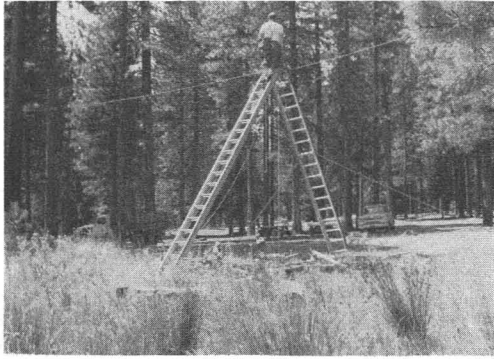
FIG. 6. A terrestrial camera station from which photographs were taken analogous to those of Figure 5. The sole purpose of erecting this station was to permit the taking of additional photography which would simulate that taken from the air. In this way several parameters involved in deriving aerial photo specifications could be investigated without the need for additional flights in a helicopter. It was possible to take the terrestrial photos more quickly, more economically and under more carefully controlled conditions. The camera station shown here was erected in less than 15 minutes. It consisted simply of two extension ladders supported in place by ropes to nearby trees and to stakes driven in the ground. For examples of the photography taken from this station, see Figures 7 and 8.
