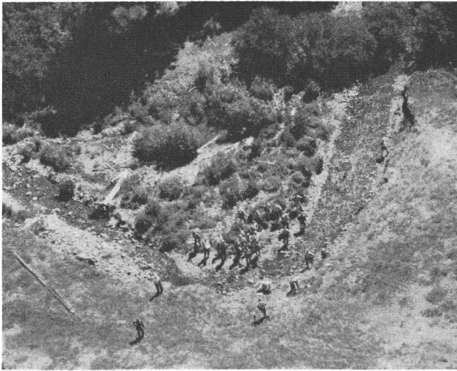
FIG. 2. Low-altitude aerial oblique photo showing the ease with which recreationists can be located and counted on large-scale aerial photography when they are not obscured by overhanging vegetation. Note in this example that photo interpretation of shadows can be of great value in differentiating between recreationists and other features. If "down-sun" oblique photos had been taken, or if the shadows had been diffused by an overcast sky, interpretation would have been much more difficult.
