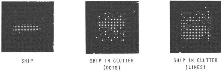
FIG. 4B. Pictures showing how (A) in Figure 4A and combinations of (A) with (B) and with (C) appear after quantization by the Mark I Perceptron Retina. These are the visual data which actually enters the machine and upon which its decisions are based.
