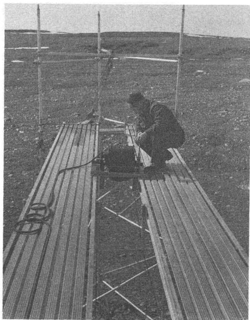
FIG. 6. Precision mapping camera and mount in position on scaffolding.
