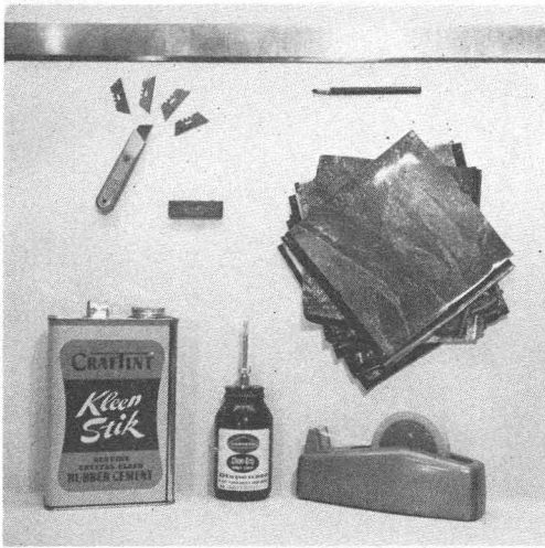
FIG. 1. Construction materials: metal straight edge, grease pencil, knife, whetstone, rubber cement and dispenser, masking tape, cardboard and photos.
