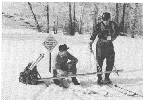
FIG. 3A. The sampling tube and snow course marker.
