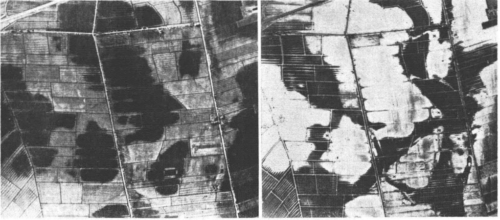
FIG. 9. The danger of relying on photographic tone measurements without due regard to seasonal state is illustrated by these two photos of an area in the central Netherlands. That which is light-toned on the left view is dark-toned on the right view, and vice-versa, even though both photos were taken with the same film-filter combination. The left photo was taken on November 29 at a time when drainage conditions in this area were very poor because drainage pumps were not working and the shallow depressions were almost flooded. The right photo was taken on the following January 5 after a heavy frost. In this photo the depressions are white, but on the low ridges the ice or snow has melted; consequently the ridges are wet and appear in dark tones. (Photos courtesy Dr. P. Buringh.)
