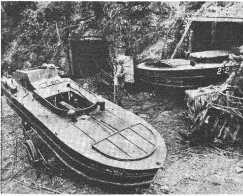
FIG. 5. Two "suicide boats" after removal from the caves in which they had been hidden. Only by identification of the objects shown in Figure 4 might the presence of these important weapons of war have been detected. Each carried a "warhead" containing 640 pounds of high explosive. (Department of Defense photo.)
