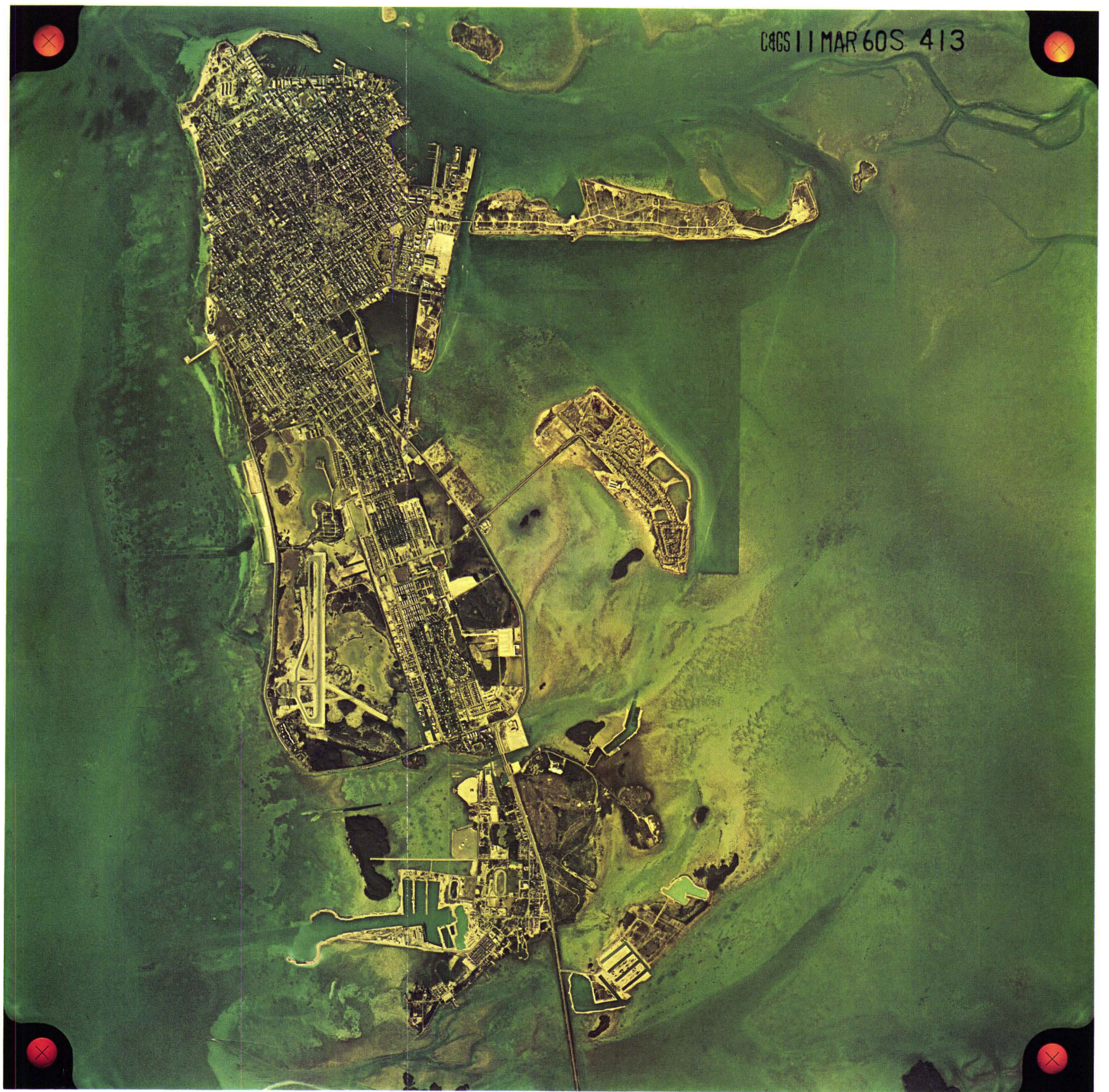
FIG. 3 All of Key West, Florida, and the surrounding area, showing both natural and man-made underwater features, are revealed in this 1:40,000 scale photograph made in March, 1960.
