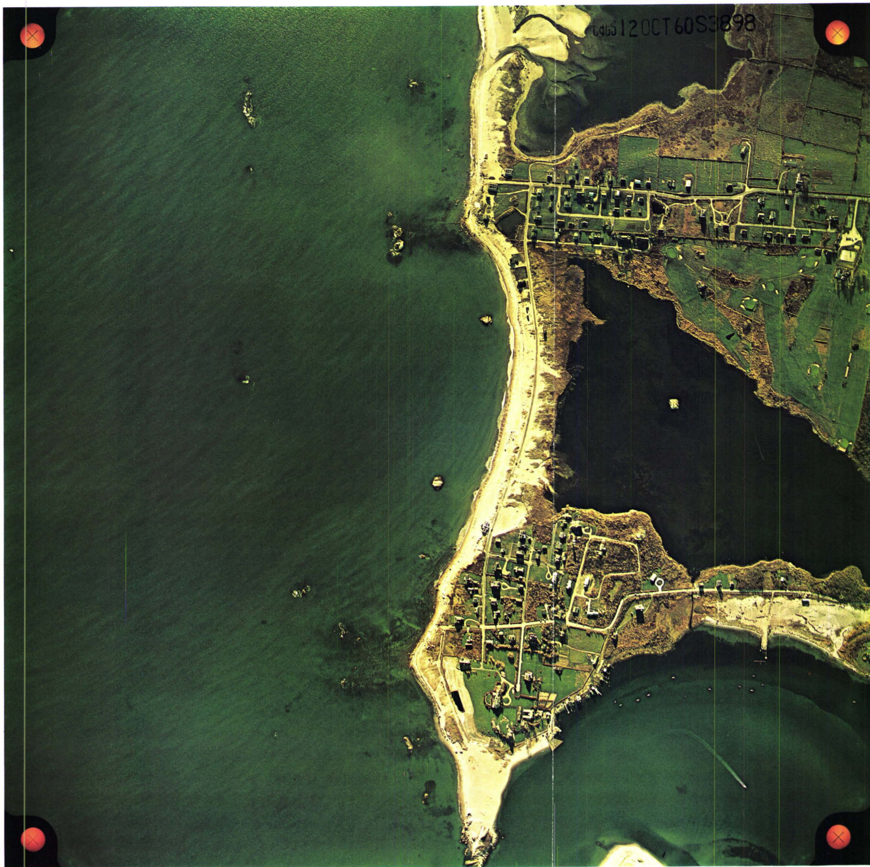
FIG. 4 Hyannis Port, Massachusetts, photographed October 12, 1960, 1:5,000 scale clearly showing water line details that are measurable when stereo pairs are viewed.
