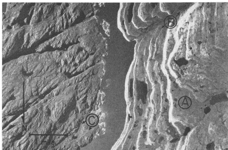
FIG. 1. Eastward dipping limestone overlies gneiss on Simpson Peninsula, Keewatin. Raised beaches are outstanding on the limestone but not on the gneiss. The medium-gray tone indicates varied vegetation (A) but grassy, wet solifluction stripes are at (B). Water and soils with a high percentage of fines are found behind the beaches because the dipping bedrock prevents adequate drainage. Sand and gravel in the gneiss area is available at (C). (Photograph courtesy R.C.A.F.)
