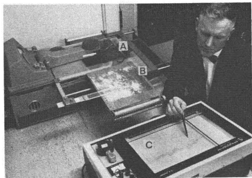
FIG. 4. Densitometer and recorder: (A) stable base film transparency, (B) stable base print for recording location of traverse, and (C) curve showing photographic density along traverse.
