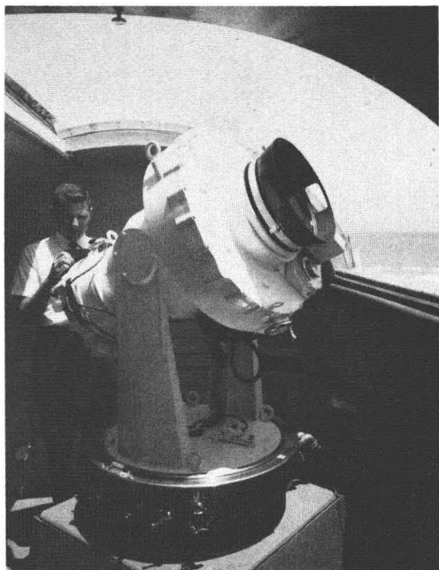
FIG. 7. Sheltered Nortronics BC 600 mm. f/2 system installation at Vero Beach.
