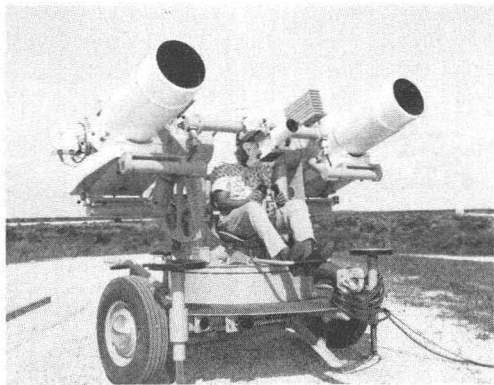
FIG. 3. IFLOT power tracking mount carrying 80 inch metric attitude cameras.
