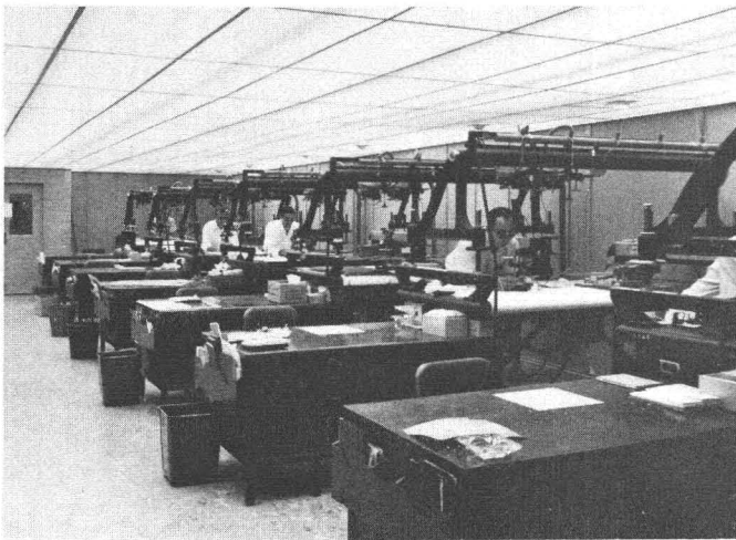
FIG. 3. A portion of experimental room containing 17 ER-55 stereoplotting instruments.
