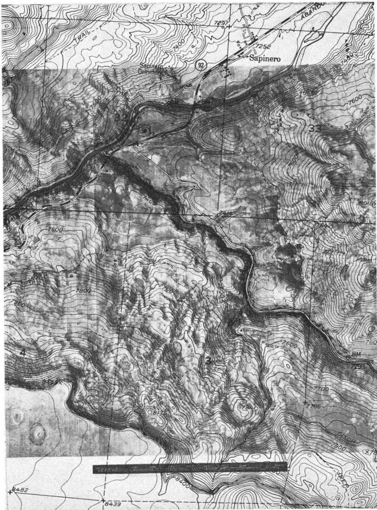
FIG. 1. A section of an orthophotomosaic of the Black Canyon of the Gunnison River, Colorado, with a superimposed transparency of a topographic map; original scale 1:24,000.
