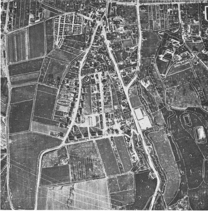
FIG. 9. Section of an orthophotomap made with the Gigas-Zeiss Orthoprojector. Original scale 1:5,000. (Zeiss-Aerotopograph photo.)
