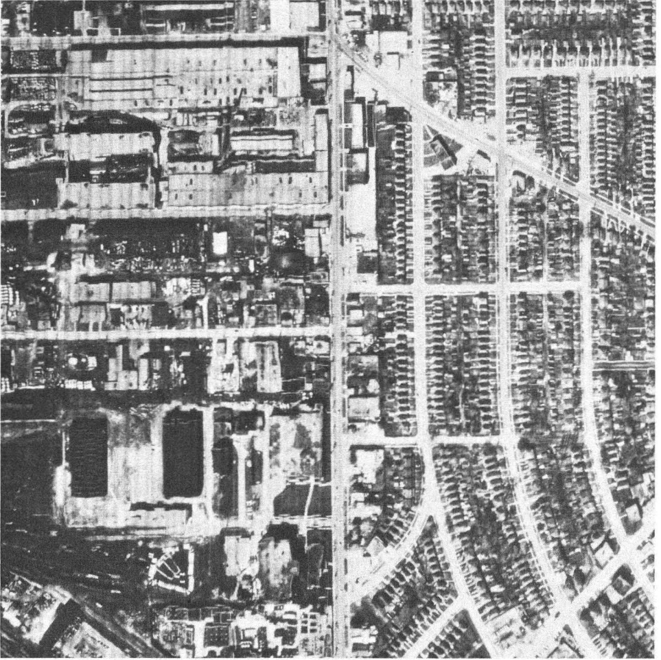
FIG. 7. An orthophotograph produced automatically with the Wild B-8 Stereomat. The original scale was 1:3,000. (Courtesy of Autometric Operation, Raytheon Co.)
