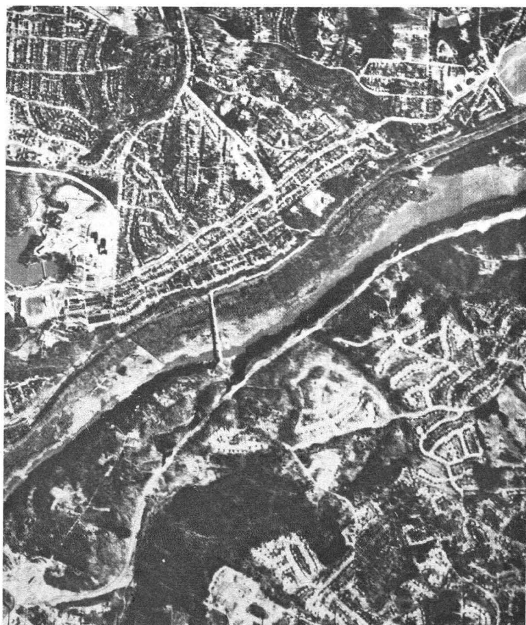
FIG. 4. Section of an orthophotomap of the Chain Bridge area on the Potomac River, original scale 1 inch equals 2,000 feet. The original was flown at 30,000 feet with a camera having a focal length of 6 inches.
