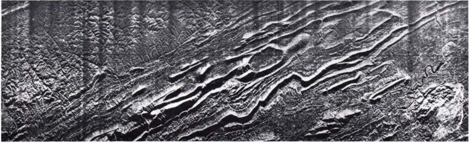
FIG. 7. Sample of radar imagery from aircraft. This imagery is several years behind the current state-of-the-art. Radar imagery reveals many earth and planetary surface features not detected by conventional photography. This radar imagery is of the Appalachian disturbed belt in Virginia. Note the position of the Burkes Garden Dome near the center of the picture.
