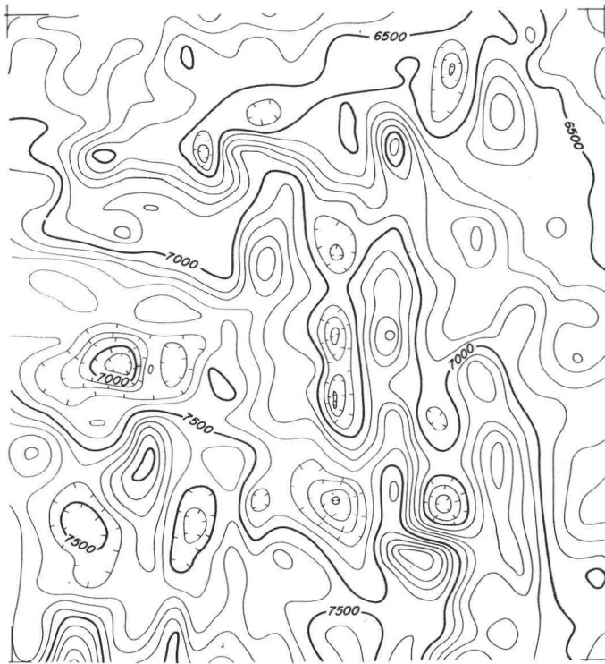
FIG. 11. Ranger Refined Compilation. Stereoplanigraph scale—1:1,000,000; X, Y-plotter scale—1:150,000; contour interval—100 meters; mesh network—900×900 meters. This compilation, not on the Selenodetic datum, was run for the purpose of testing the programs in the total ATC system.
