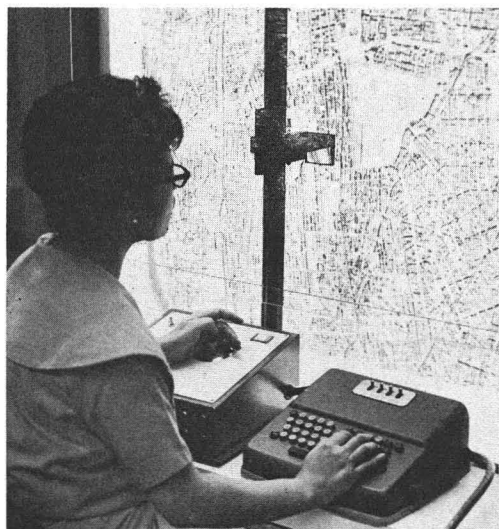
FIG. 4. Operator seated at AULT Reader looking through reading head at point on photomosaic, with left hand operating the joy-stick of the control box and right hand on the keyboard.
