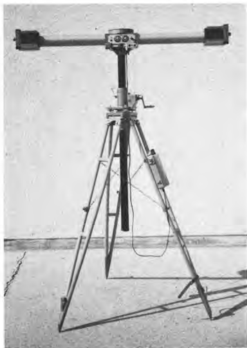
FIG. 1. Stereometric Camera Wild C120 showing the control panel.
