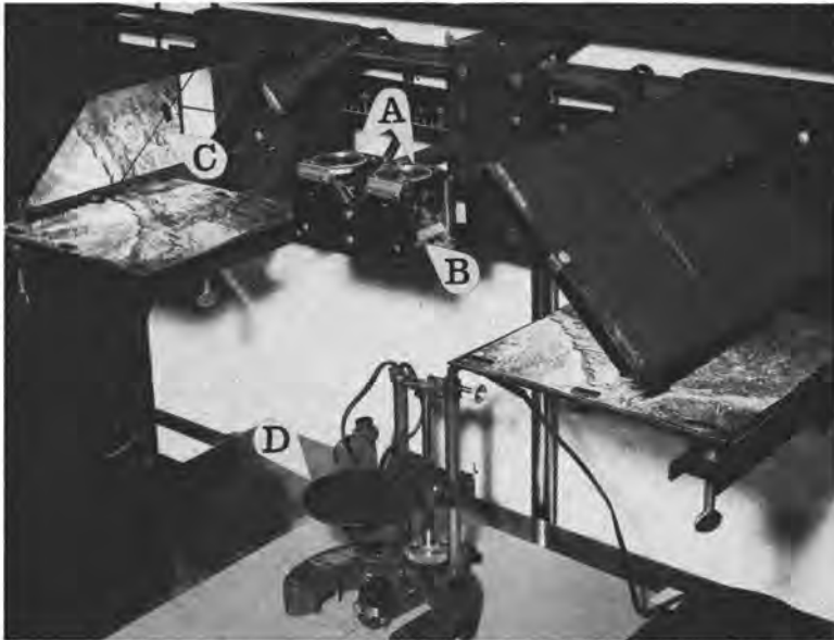
FIG. 2. A close-up view of the Multiscope with recommended modifications. New holders for the diopter viewing lenses at A provide for a greater field of view than is possible with original instrument design. Spring-loaded adjustable mounts were added to each of the half-silvered mirrors (one is shown at B) to facilitate optical calibration of the instrument. A thread, aligned over the center of each wing mirror and in the X-direction of the instrument, has been added (see C) to provide a reference line for rapidly aligning the centers and conjugate centers of each photograph. This thread also reduces errors resulting from parallax displacement, as these lines are vertically above the photo plates and any movement of the head in a backward or forward direction is readily apparent in the stereoscopic model. Because it is necessary to see only the illuminated dot of the Multiplex tracing table in the stereoscopic model, and because the white surface of the tracing table (platen) causes a diffusion of the stereoscopic imagery, the table is painted black (see D).
