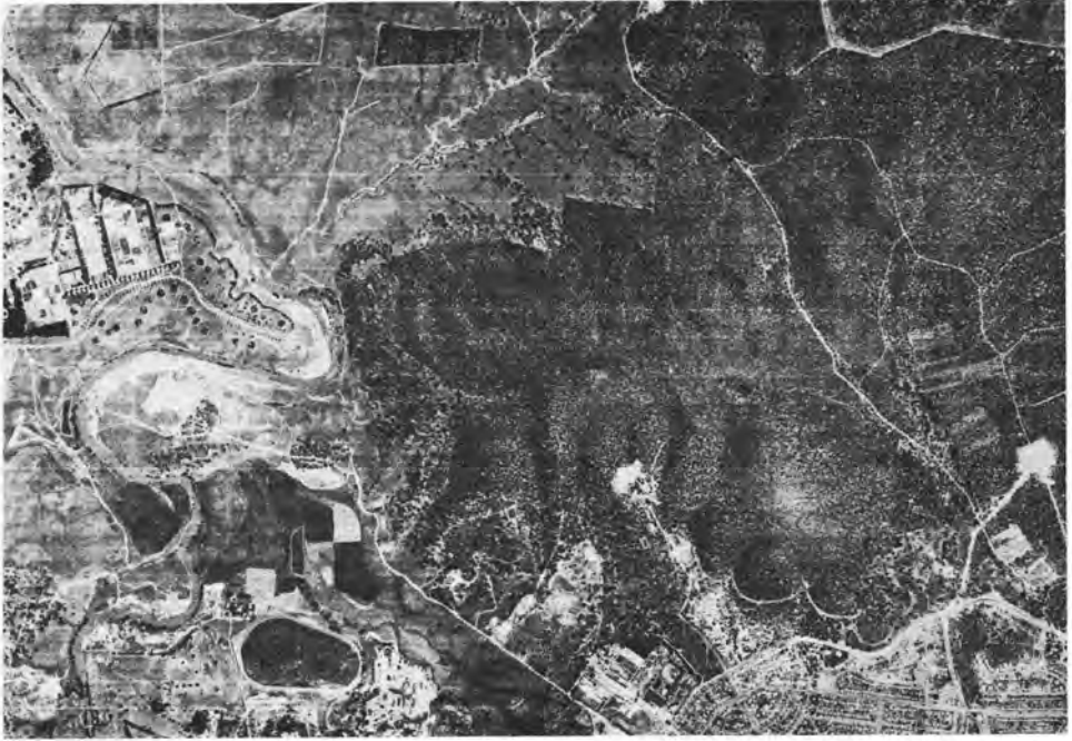
FIG. 18. Orthophotograph 1:31,680 (before reduction), produced from super-wide-angle air photographs 1:74,400. By courtesy of Dept. of National Mapping, Canberra.
