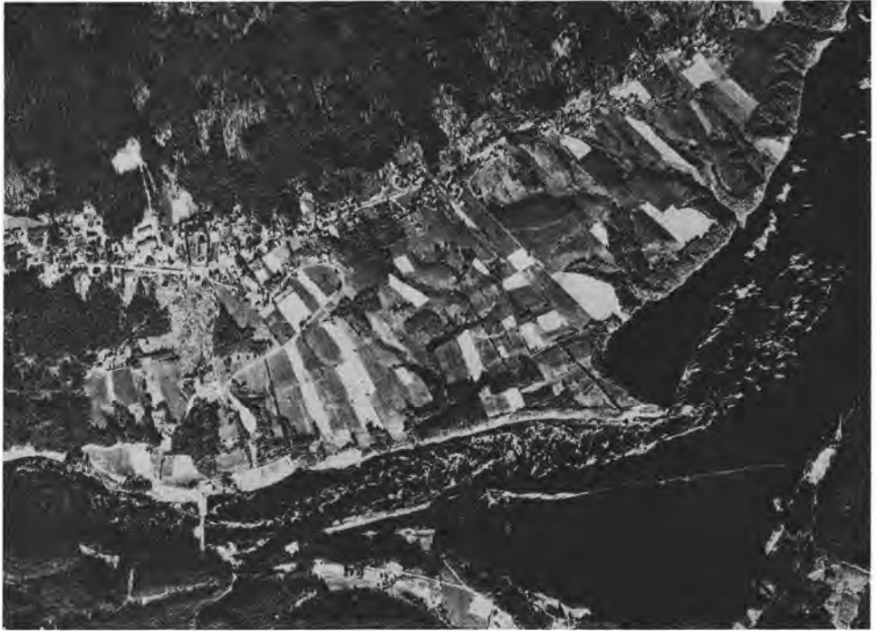
FIG. 12. Orthophotograph 1:10,000 (before reduction), produced from wide-angle air photographs 1:30,000. (The illustration is a reduction of 0.45.) By courtesy of Rikets Allmana Kartverk, Stockholm.
