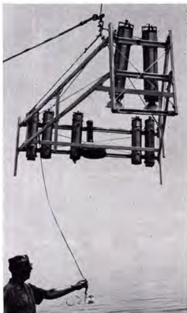
FIG. 6. A-frame configuration Model B of a deep-sea camera being lowered over the side.
