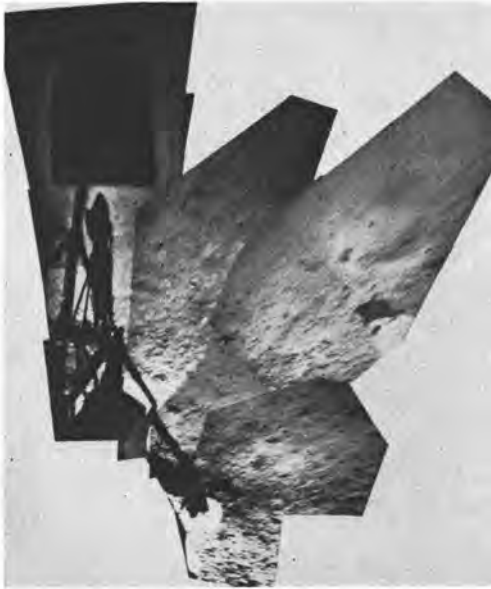
FIG. 6. Rectified mosaic of wide-angle pictures taken by Surveyor I. The prints were made with a projector from the Surveyor stereoplotter.
