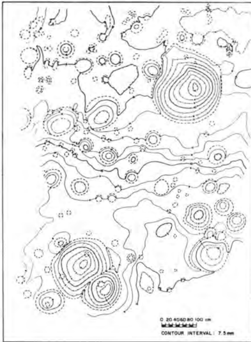
FIG. 3. Contour map of the surface model compiled with the Surveyor stereoplotter and pictures in Fig. 2. Physical measurement of the model showed that the map datum was tilted a total of 40 minutes along its greatest dimension, and after adjusting for this tilt, most elevations interpolated from contour lines were found to be accurate within \pm 4 mm.
