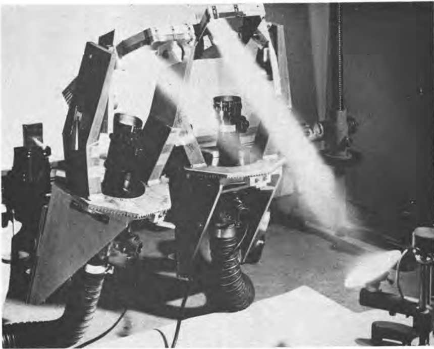
FRONTISPIECE. Prototype Surveyor stereoplottor. Each projector is a geometric analog of the Surveyor television camera. Glass diapositives approximately 11 \times 11 mm. are used in the projectors, and the stereoscopic model can be viewed on the platen of a conventional tracing table.
