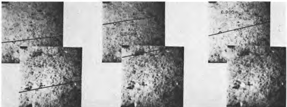
FIG. 7. Pictures from Surveyor I focus-ranging survey. Saw-toothed lines enclose the areas of best focus for the focus settings noted on the pictures.
