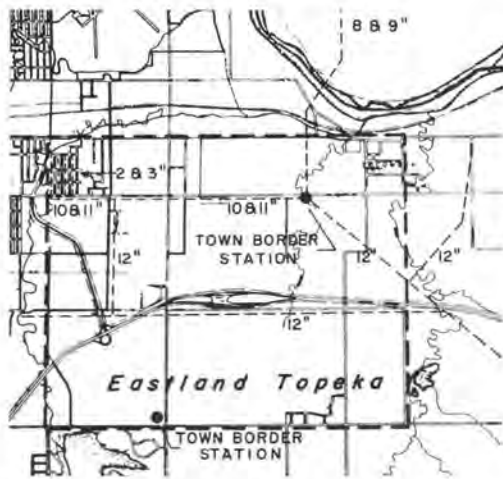
FIG. 13. Existing gas mains as of January 1962.
