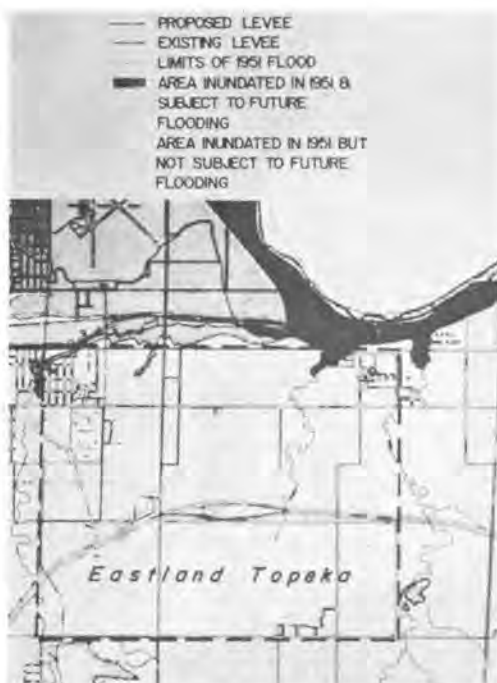
FIG. 8. Map of the Eastland Topeka area showing the flood plain including existing and proposed levees.
