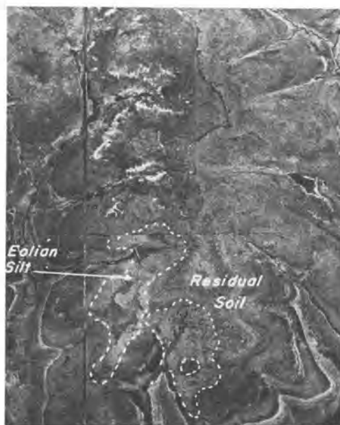
FIG. 3. An aerial photograph of an area in central Kansas portraying eolian silt deposits. In this area, residual soils are portrayed in a "banding" pattern corresponding to the underlying sedimentary rocks. The eolian silt is delineated by tonal changes and a distinctive gully pattern which develops in the deeper deposits.
