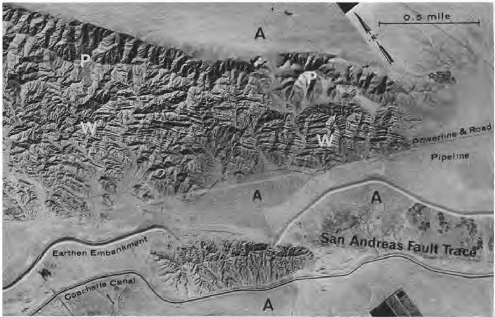
FIG. 4. Vertical aerial photograph of the southeast end of Indio Hills. Compare with the lower strips of imagery in Figures 2 and 3. See Figure 2 for the explanation of the stratigraphic-radiometric units.
