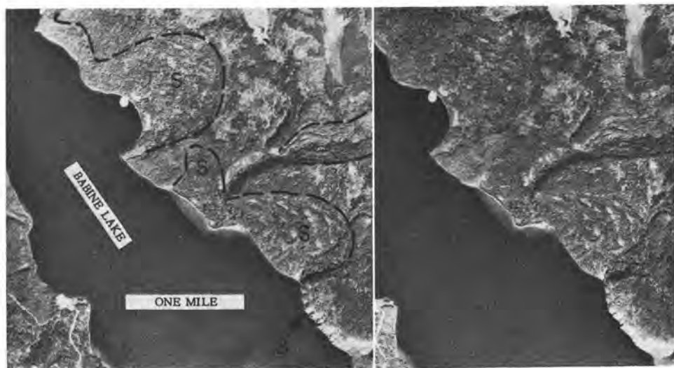
FIG. 1. Massive slumps and earth flows S have occurred in deep glacial materials on the north side of Babine Lake in British Columbia. A nearby bluff of columnar basalt B shows no sign of instability. Deep glacial materials consist of glacial till and lakebed sediments. These materials were deposited against glacier ice which occupied Babine valley during melting of the glaciers. Canadian Government Airphoto.
