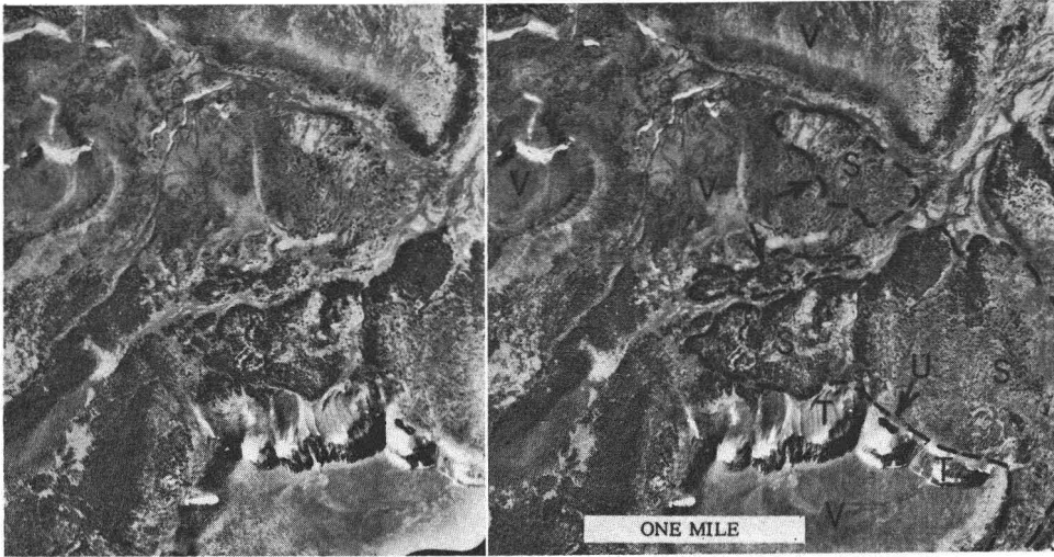
FIG. 6. Mount Downton (7760 ft.), an extinct volcano in the interior of British Columbia was deeply eroded by glaciers during the last Ice Age. Bedrock slumps S occurred when glacier ice melted out of U -shaped valleys. Scarp faces with associated talus T and undrained ponds U help to identify sites of massive slides. Unfailed volcanic bedrock V has been well rounded by glacial erosion. Canadian Government Airphoto.
