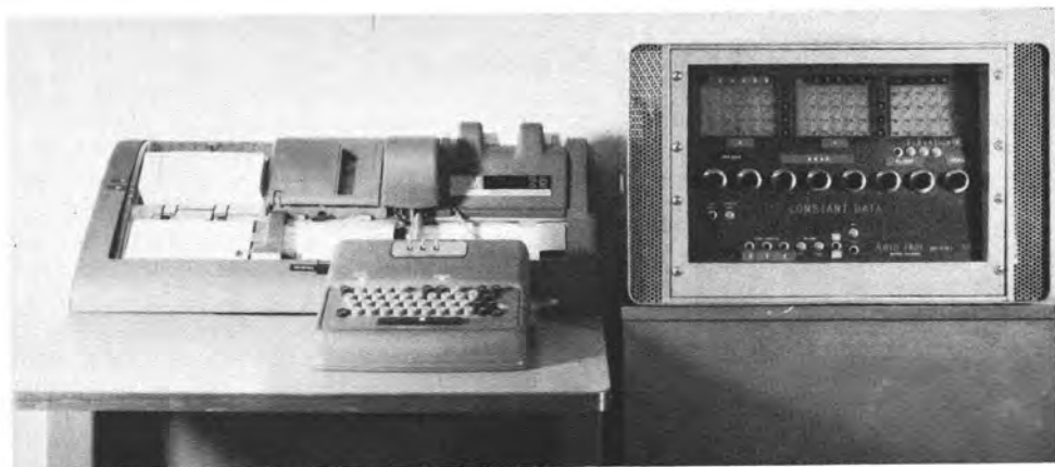
FIG. 5. On the left is an IBM Printing Card Punch adapted for dip identification and x -, y -, z -coordinates. On the right is the Analog-to-Digital converter designed by Auto-Trol Corporation.
