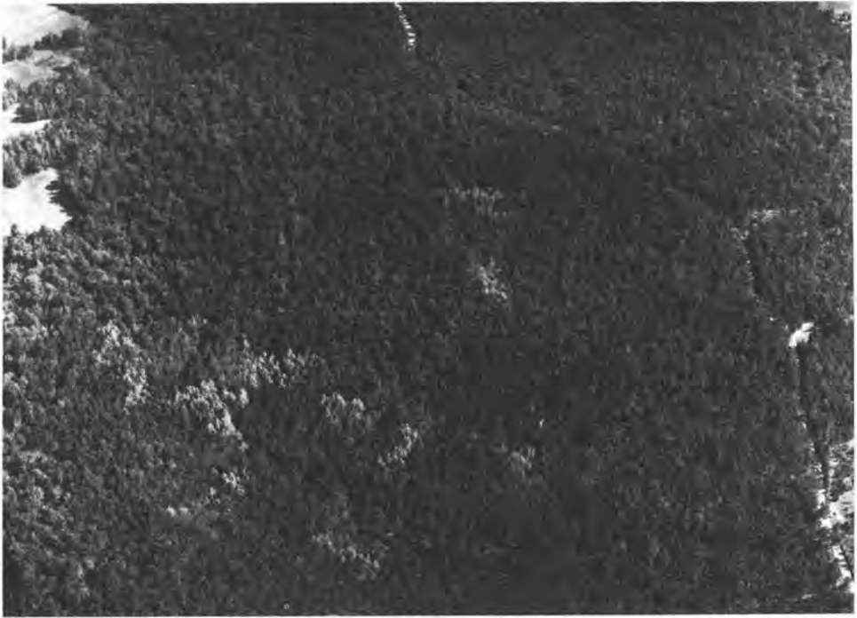
FIG. 5. Intermediate resolution of features by black and white photography taken from several thousand feet above the terrain can provide satisfactory detection of insect attacks to standing timber. Here the light-toned trees are southern pines killed by bark beetles in Mississippi. This kind of imagery is also useful for planning control of forest pests and timber salvage. (U. S. Forest Service Photograph.)
