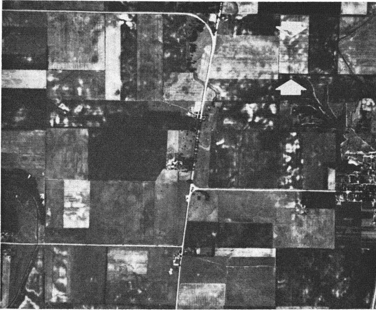
FIG. 3. Area of Tinley ground moraine, northeastern Dupage County. Mottled appearance is generally characteristic of tills in the midwestern United States. Arrows indicate one (and possibly two) fracture traces trending N 5°E.
