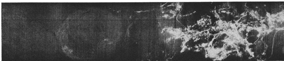
FIG. 5. Infrared imagery of the Norris Geyser Basin and Gibbon Hill, Yellowstone National Park. Gibbon Hill is shown as a nearly round thermal anomaly in the right portion of the strip. The imagery portrays a strip one mile wide.
