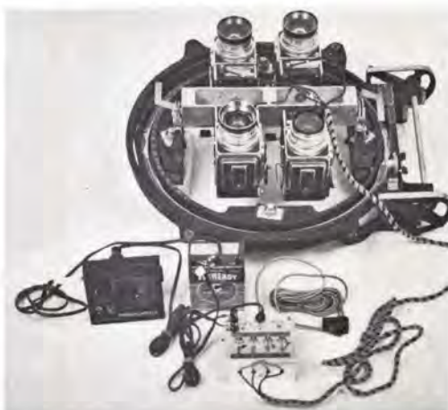
FIG. 5. The assembled system of cameras, mount, and controls. The unit below the cameras and to the left is the Nikon Intervalometer. To the right of it is the battery and next to it is the manual trip cable. Below them is the control box.
