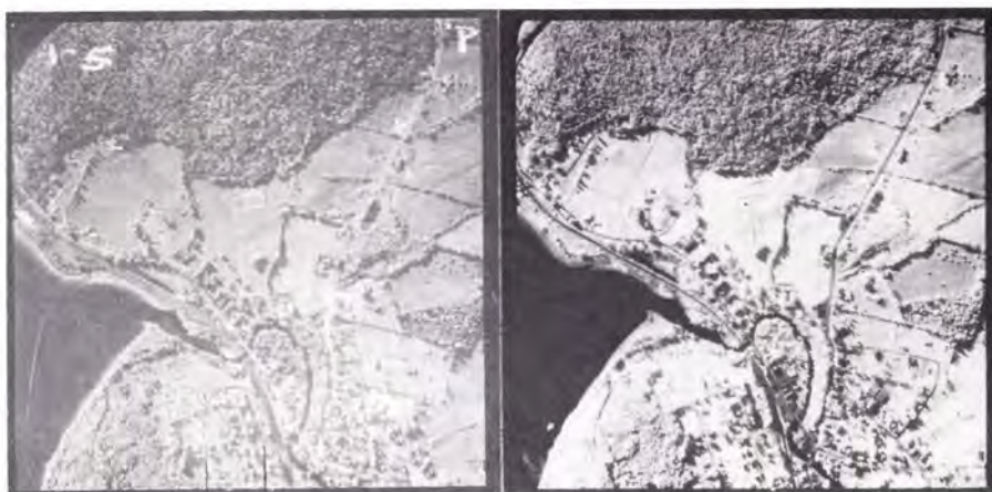
FIG. 6. Photographs of an area in New Hampshire (October 1966) taken on Tri-X film (left) and Gevaert I. R. film (right) with an 80-mm lens (approximate scale, 1:28,000).
