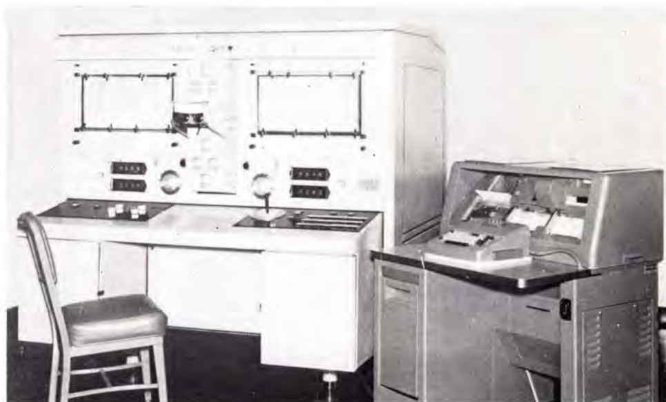
FIG. 1. The Variscale Stereo Point Marking Instrument manufactured by Bausch & Lomb, Inc. for GIMRADA.
